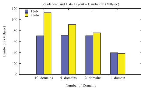
Fig. 8. The impact of ill-mapped data layout for readahead with queue depths of one and eight jobs.
